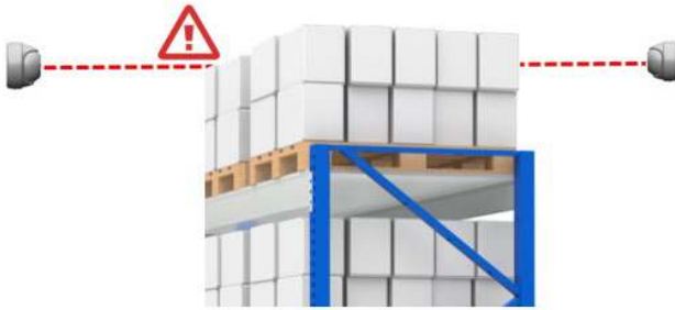
Beam detectors blocked by objects
