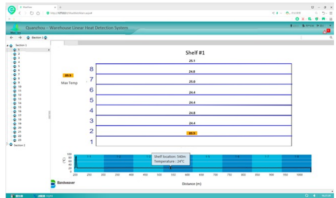
Figure 12 – Screenshot profile view of rack 1 within warehouse
